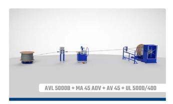
Whether our customers are handling high volumes with low variability or a more challenging product variation, we can integrate systems that reduce labour and increase product quality. For smaller and mediumsized wire ropes we offer integrated machine packages that manage the measure-cut-coil process either semi automatic or fully automatic.
